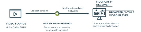
Each viewing device on the network, such as a personal computer, hosts a Multicast+ Receiver. The Receiver makes the client capable of tapping into multicast broadcast streams. When video streams are received, they are unencapsulated and made available locally to the browser, the same way the browser would receive content from any web server.
